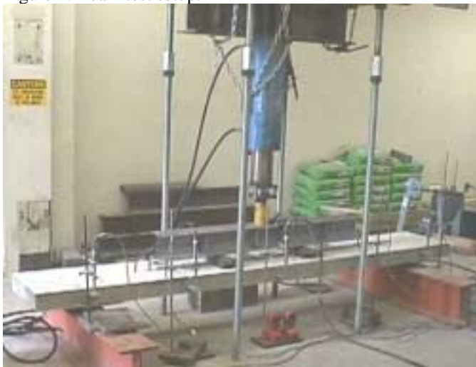
Figure 3: Slab test setup.
