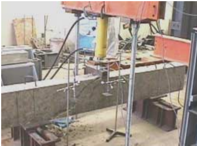
Figure 2: Beam test setup.
