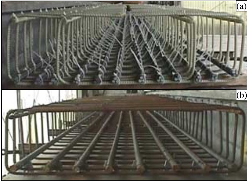
FIGURE 1 FRP and steel reinforcement layouts.
