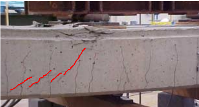
FIGURE 5 Failure of the FRP-RC panel during the flexural testing.
