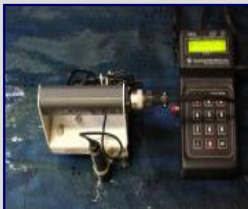
Echo-Impact NDT of Delaminations
