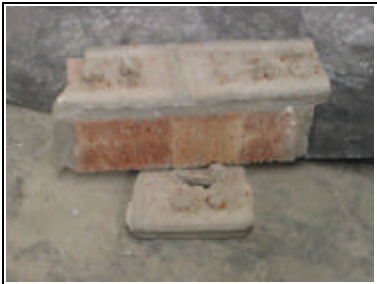
Figure 14. Dowel action effect
