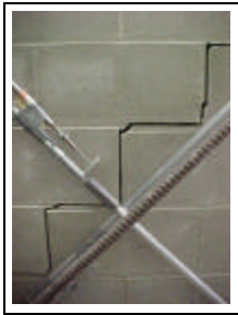
Figure 7. Star shape behaviour in one-side reinforced walls
