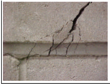
Figure 11. Crack Behaviour in one side (left) and two-sides (right) reinforcement
