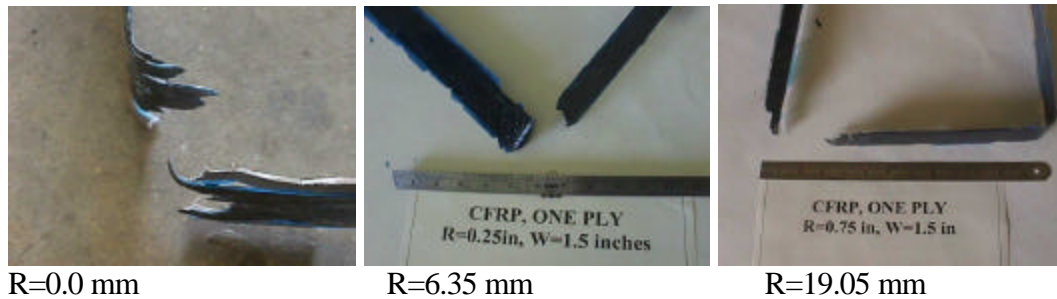
Fig. 7 Failure modes of CFRP laminates
