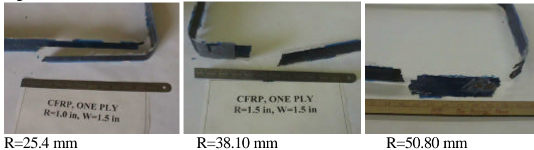
Fig. 7 Failure modes of CFRP laminates
