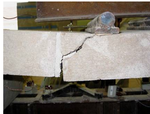
d) Flexural – Shear Failure (CO2-GRC33)
