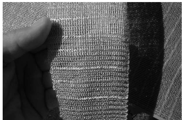
Fig. 4. Cords held together by two knit yarns made from polyester.
