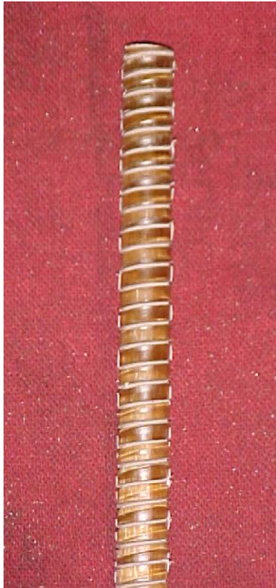
Fig. 2. Threaded end to improve anchorage.
